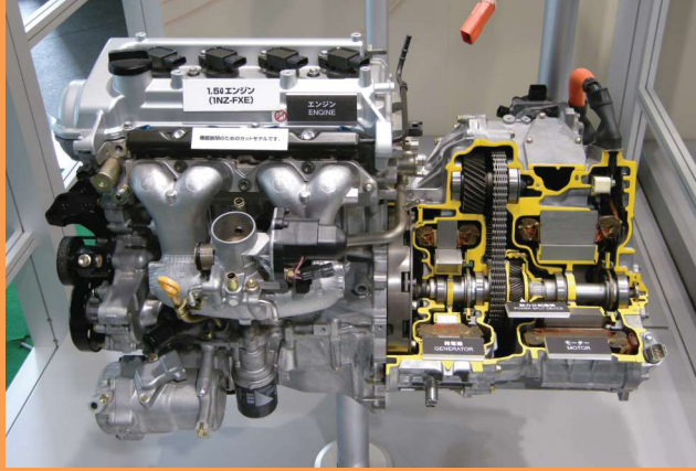
Fig. 5. Assembly of system: ICE (left); MG1 and MG2 connected in E-CVT (right)
